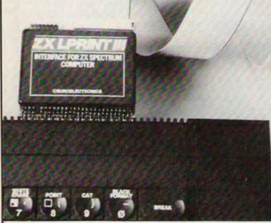
ZXLprint III interface enables your Spectrum computer (16 or 48K) to print on almost any dot matrix or daisy wheel printer with RS232 or Centronics input. Just plug in ZXLprint III and LPRINT and LLIST commands will work. COPY works without any software on Epson, Star Delta, Brother HR5 & 1009, Gemini, Walters WM80, Mannesman MT80, Kaga Taxan, Cannon, Shinwa, Seikosha 100, 250 & 500. Plus Seikosha GP700 in FULL COLOUR. Also available is optional COPY in 4 colours on CGP115, MCP40 & 80 and SCP80.
