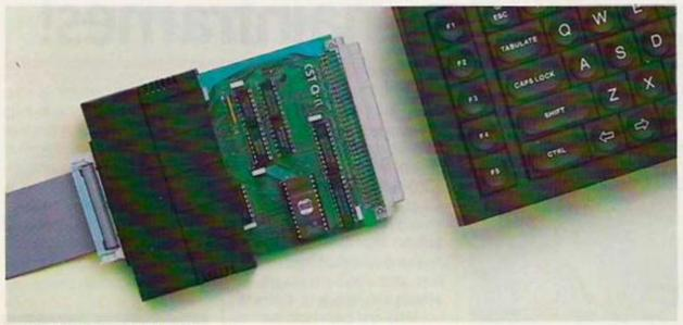
An IEEE-488 interface slips discreetly into place.
